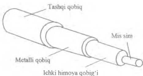
6.2-rasm. Koaksial kabel tuzilishi.
