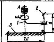
**12.2.3.** 1 disk ikkita aylanma harakatda ishtirok etadi. Birinidan disk 2 dastak o'z o'qi atrofida  $300\text{ayl/min}$  chastota bilan, 2 dastak esa 3 podshipnik atrofida  $\omega_2=10\text{rad/s}$  burchak tezlik bilan aylanadi. Diskning absolut burchak tezligini toping. (33,0)
