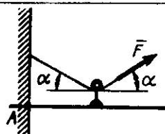
**2.4.41.** Yerga qistirib mahkamlangan, uzunligi  $AB=5,66\text{m}$  bo'lgan to'sinning uchiga  $F$  kuchi ta'sir etayotgan bo'lsa, A tayanchdagi reaksiya momenti  $M_A=56\text{kN}\cdot\text{m}$  ga teng bo'lsa,  $F$  kuchining qiymatini  $\text{kN}$  da toping. (14,0)
