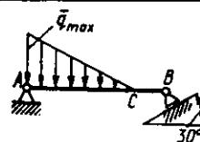
**2.4.9.** O'lchamlari  $AB=BC=3\text{m}$ ,  $CD=1\text{m}$  bo'lgan  $AD$  to'singa momenti  $M=13\text{kN}\cdot\text{m}$  li just kuch va intensivligi  $q_{\max}=8\text{kN/m}$  li taqsimlangan kuchlar ta'sir etsa,  $D$  tayanch reaksiyasini kN da hisoblang. (10,0)
