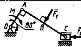
**3.3.10.** Kulisali mexanizm  $F_1=1\text{kN}$  va  $\bar{F}_2$  kuchlar ta'sirida muvozanat holatida bo'lib,  $OA=0,5\text{m}$ ,  $OB=1,2\text{m}$ ,  $\varphi=30^\circ$ ,  $\alpha=60^\circ$  bo'lsa, 1 vtulkaning 2 vertikal sterjenga bosim kuchini kN da aniqlang. (2,08)
