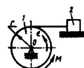
**17.3.17.** Vibrator ikki sinxron aylanuvchi pnevmoturbinalardan iborat bo'lib, ularning valiga  $r=10\text{sm}$  masofada  $m=0,5\text{kg}$  massalar o'rnatilgan. Agar tribinalar  $n=1000\text{ayl/min}$  chastotasi bilan aylansa, vibrator asosiga ko'rsatilayotgan eng katta dinamik zo'riqishni toping (kN). (1,10)
