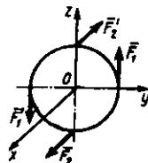
**5.2.12.** Mashina detalining to'rt tomoniga miqdorlari teng  $M_1=M_2=M_3=M_4=5\text{N}\cdot\text{m}$  momentli juft kuchlar va  $Oyz$  tekisligida qiymati  $\bar{F}=\bar{F}'=100\text{N}$  bo'lgan ( $\bar{F}, \bar{F}'$ ) juft kuch ta'sir etsa, juft kuchlar sistemasining teng ta'sir etuvchisining momentini toping. Bunda  $a=0,05\text{m}$  va  $\bar{F} \parallel Oz$   $\bar{F}' \parallel Oz$  deb oling. (17,3)
