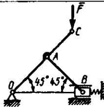
3.3.8. Krivoship-polzunli mexanizm  $F_1=1$  kN va  $F_2$  kuchlar ta'sirida muvozanatda bo'lsa,  $OA=AC=0,3$  m va  $\alpha=45^\circ$  deb,  $OAC$  krivoship va  $AB$  shatunning o'zaro ta'sir kuchini kN da aniqlang. (1,41)
