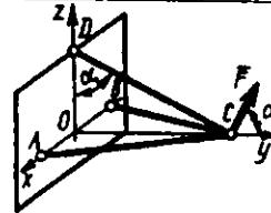
**1.4.4.** Uchta sterjen  $AD$ ,  $BD$  va  $CD$  sharnirlar bilan mahkamlangan bo'lib,  $D$  sharniriga  $20\text{N}$  li yuk osilgan bo'lsa,  $CD$  sterjening zo'riqishini toping ( $\alpha=45^\circ$ ). (-28,3)
