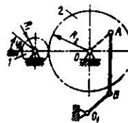
8.4.14. Radiuslari  $R_1=0,3\text{m}$ ,  $R_2=0,9\text{m}$  bo'lgan tishli g'ildiraklarga bog'langan krivoshipning o'lchamlari  $O_1M=0,3\text{m}$ ,  $OA=O_1B$  va  $AB=OO_1$  bo'lib, 1 g'ildirak o'zgarmas  $\omega_1=6\text{rad/s}$  burchak tezlik bilan aylansa, krivoship M nuqtasining tezlanishini toping. (1,2)
