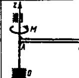
**16.1.16.** Dvigatel rotoriga  $M=100(1-\omega/200)$  juft kuch momenti ta'sir etib, uni ishga tushirsa, rotoring inersiya momentini  $2\text{kg}\cdot\text{m}^2$  hisoblab, rotor burchak tezlanishining maksimal qiymatini aniqlang. (50)
