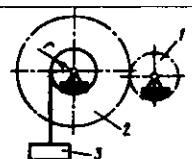
8.4.11. Radiuslari  $R_1=1\text{m}$ ,  $R_2=0,8\text{m}$  va  $r_2=0,4\text{m}$  bo'lgan pog'onali g'ildiraklarga 3 yuk osilgan. Agar 1 g'ildirakning burchak tezligi  $\omega_1=2t^2$  berilgan bo'ssa,  $t=2\text{sda}$  3 yukning tezlanishini aniqlang. (4)
