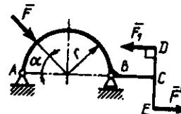
**2.1.8.**  $AB$  arkaga ( $\bar{F}_1$ ,  $\bar{F}'_1$ ) juft kuch va  $F$  kuchi ta'sir etadi. Agar kuchlarning miqdori  $F=4\text{N}$ ,  $F_1=2\text{N}$ , arka radiusi  $r=2\text{m}$ , juft kuch yelkasi  $CD=1,5\text{m}$  bo'lsa, ularning  $A$  nuqtaga nisbatan momentlarining yig'indisini aniqlang. (-11,0)
