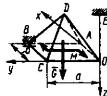
**5.6.10.** O'lchamlari  $a=20\text{sm}$  bo'lgan bir jinsli plita  $G=400\text{N}$  og'irlikka ega. Agar plita shaklda ko'rsatilgan bog'lanishlar vositasida muvozanatda bo'lib,  $\alpha=61^\circ$ ,  $\beta=44^\circ$  va  $\gamma=60^\circ$  bo'lsa,  $AB$  arqonning taranglik kuchini,  $Ox$  o'qiga nisbatan moment tenglamasini tuzib toping. (400)
