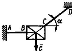
**1.2.13.** Ikki sterjen  $AC$  va  $BC$  o'zaro  $C$  sharnir yordamida bog'langan. Agar  $C$  sharniriga  $D$  blok orqali og'irligi  $12\text{N}$  bo'lgan yuk osilib,  $\alpha=60^\circ$  bo'lsa,  $BC$  sterjenning reaksiya kuchini toping. (-6)
