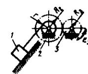
8.4.13. Radiuslari  $R_1=0,3\text{m}$ ,  $R_2=0,9\text{m}$  bo'lgan tishli g'ildiraklarga mahkamlangan krivoshipning o'lchamlari  $O_1B=OA=0,6\text{m}$  va  $OO_1=AB$  bo'lib, 1 g'ildirak  $\varphi_1=2t^3$  qonun bo'yicha aylansa,  $t=2\text{s}$  paytda krivoship B nuqtasining tezligini aniqlang. (4,8)
