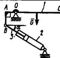
**2.4.31.** Avtornashininining kuzovi  $G=10\text{kN}$  og'irlikka ega bo'lib, 2 kuch gidrosilindr yordamida muvozanatda ushlab turibdi. Agar masofa va burchaklar  $\ell=3\text{m}$ ,  $b=1,2\text{m}$ ,  $AO=1\text{m}$ ,  $\alpha=30^\circ$  bo'lsa, gidrosilindr 3 dastagiga ta'sir etuvchi kuchni aniqlang. (11,5)
