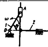
**14.1.16.** Krivoship-polzunli mexanizmning  $A$  va  $B$  nuqtalarining tezlanishi  $a_A=10\text{m/s}^2$  va  $a_B=14\text{m/s}^2$  bo'lib, massasi  $m=5\text{kg}$  bo'lgan, bir jinsli sterjen shaklidagi shatun  $AB$  ga ta'sir qiluvchi tashqi kuchlar bosh vektorining  $\varphi=180^\circ$  holatdagi miqdorini toping. (60)
