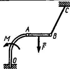
**3.2.3. O'lchamlari  $AB=2\text{m}$  va  $BC=0,5\text{m}$  bo'lgan sterjenlardan iborat sistemaga momenti  $M=800\text{N}\cdot\text{m}$  li just kuch ta'sir etsa,  $C$  tayanchdagi reaksiya momentini aniqlang. (200)**
