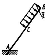
**2.4.49.** Devorga qistirib mahkamlangan rama-ga  $F=150\text{N}$  kuch va intensivligi  $q_{\max}=40\text{N/m}$  bo'lgan taqsimlangan kuch ta'sir etib, to'sinning o'lchamlari  $AD=BD=1\text{m}$ ;  $BC=3\text{m}$  bo'lsa,  $A$  tayanchdagi reaksiya momentning miqdorini toping. (195)
