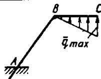
**2.3.22.** Qistirib mahkamlangan to'sinning qancha  $\ell$  qismiga intensivligi  $q_{\max}=10\text{N/m}$  li taqsimlangan kuchlar ta'sir etsa,  $A$  tayanchning reaksiya kuchi  $R_A=10\text{N}$  ga teng bo'ladi? (2,0)
