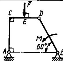
**3.2.14.** O'lchamlari  $BC=2AB$  bo'lgan  $AC$  sterjenga  $F=600 \text{ N}$  kuch ta'sir etsa,  $C$  sharnir reaksiya kuchining vertikal tashkil etuvchisini toping. (200)
