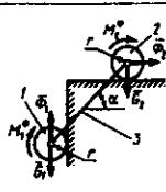
**19.3.10.** Reduktorli mexanizm just kuch momenti  $M$  ta'sirida harakatga kelib, tishlar soni  $Z_1=50$ ;  $Z_2=100$  bo'lgan shesternyalarini aylantiradi. Agar shesternyalariga inersiya kuchlarining bosh momentlari  $M_1^\Phi=0,1\text{N}\cdot\text{m}$ ,  $M_2^\Phi=1\text{N}\cdot\text{m}$  ta'sir qilsa, tasmali uzatmanning uzatish nisbati  $i=0,5$  deb, aylantiruvchi moment  $M$  ning qiymatini toping. (0,3)
