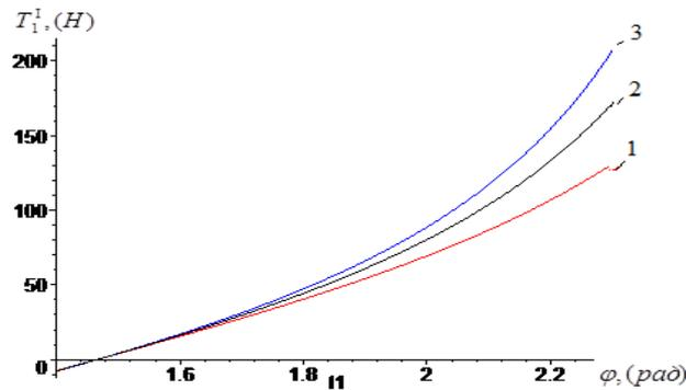
**Fig. 6.** The graph of the tension of the fiber layer at the input as a function of the coverage angle at different speeds.
