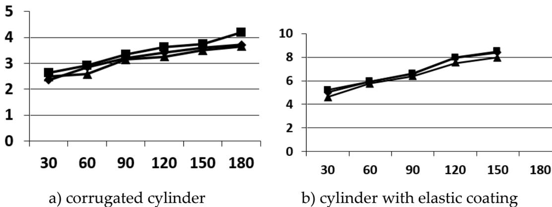
**Figure 1.** The width of the contact line in the front zone depends on the amount of load and the design of the output cylinder.
