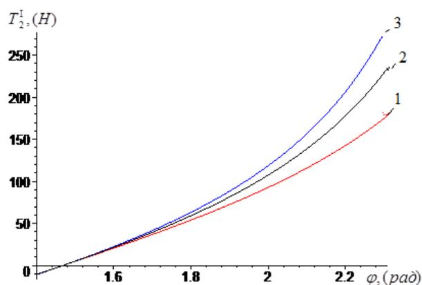
**Figure 7.** The tension of the output thread in different twists  $K_1 = 400$  twist/meter,  $K_2 = 500$  twist/meter,  $K_3 = 600$  twist/meter coverage angle graph.
