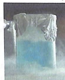
Suyuq kislorod ( T_{\text{suyuq}} = -183^\circ\text{C} )
