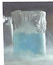
Suyuq kislorod ( T_{\text{suyuq}} - 183^\circ\text{C} )
