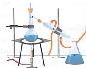
Haydash. 1-haydash kolbasi, 2- termometr, 3-sovitgich, 4-yig'gich kolba
