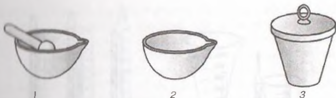
2-rasm. 1 — chinni havoncha, 2 — chinni kosacha, 3 — chinni tigel.
