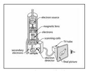
heavy metal. This enables the SEM to produce images of whole specimens: cells, tissues, or even organisms.
