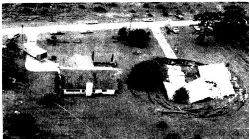
14.15-rasm. Yerosti suvlari natijasida yerning cho'kishi (Understanding Earth., J. Grotzinger va b.).
